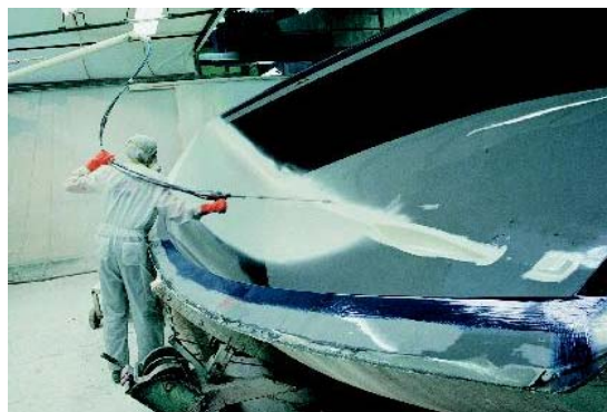
Precautions need to be taken during spraying to avoid static build-up
